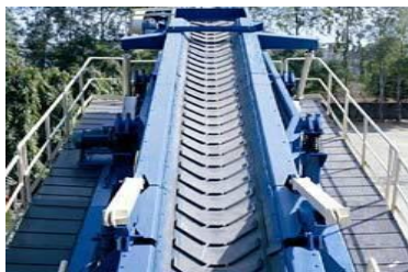
Fig.2. Example of a conveyor with limited space for the gearbox and the motor.
