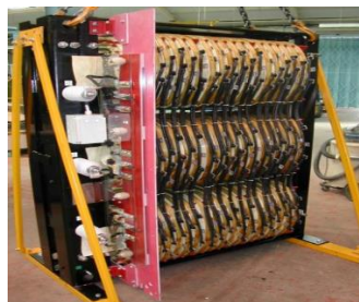
Fig.3. Transformer for SCHB converters.
