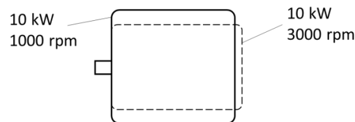
Fig.7. Sizes of the machines of the same power but of different speed.
